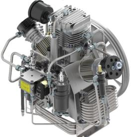
The bearings of the crankshaft have rollers, extremely robust and made in Europe which guarantee a long life of the compressor. An oil pump provides a constant lubrication of the inner workings of the block with oil cleaned of impurities by a filter and by a magnet which catches any metals present in the lubricating oil. The compressed air cooling is obtained by inter-stage stainless steel cooling coils.
