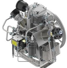
The bearings of the crankshaft have rollers, extremely robust and made in Europe which guarantee a long life of the compressor. An oil pump provides a constant lubrication of the inner workings of the block with oil cleaned of impurities by a filter and by a magnet which catches any metals present in the lubricating oil. The compressed air cooling is obtained by inter-stage stainless steel cooling coils.
