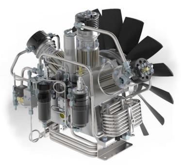
The bearings of the crankshaft have rollers, extremely robust and made in Europe which guarantee a long life of the compressor. An oil pump provides a constant lubrication of the inner workings of the block with oil cleaned of impurities by a filter and by a magnet which catches any metals present in the lubricating oil. The compressed air cooling is obtained by inter-stage stainless steel cooling coils.
